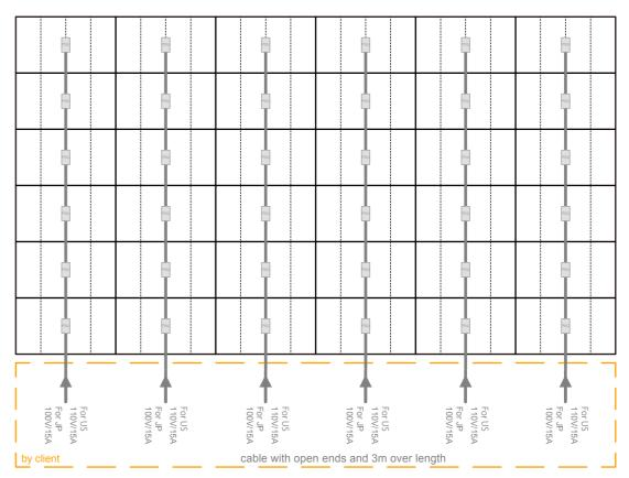
The 15A(US) or 16A (EU) circuit breaker for the each power feed must have a european D characteristic or similar. (can hold for a short term 20times the tripping current)
