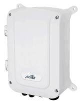
The H60 series of IP67/IK10 Pro L2 Managed PoE Switches are designed with 6KV Ethernet port surge protection, 4KV surge protection in DC Input, and hardengraded standard to operate between -40° C and 65° C for harsh weather conditions. They enable outdoor connections of PoE PDs to the network such as outdoor IP cameras, wireless APs, and other outdoor industrial applications.
