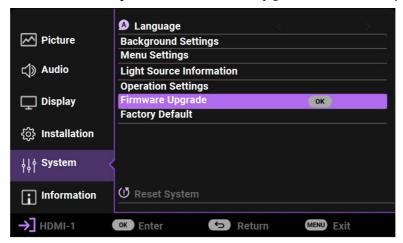
5. Select **Yes** to upgrade the firmware version. Keep the projector power on until the firmware upgrade is finished.
