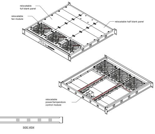
Maximum fan quantity for FTA-3 and FTA-6 is 8 when used with optional FT-FAN kits.
