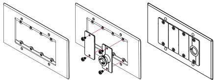
2. Connect the cable ports to the rear side of the insert(s).
