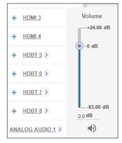
Figure 64: Port Settings –Setting Analog Audio Level
