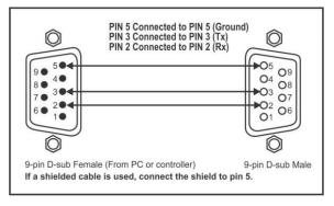
Figure 6: RS-232 Cabling Pinout
