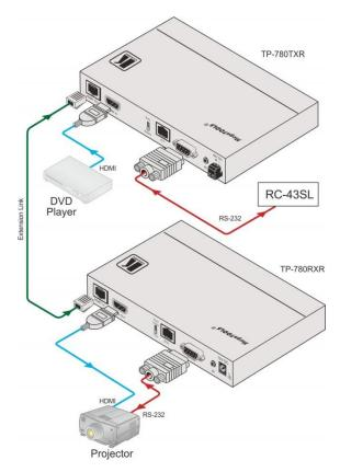
Figure 3: Connecting the TP-780TXR/TP-780RXR Transmitter/Receiver Pair
