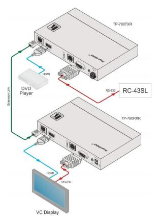
Figure 7: RS-232 Control via the TP-780TXR/RXR
