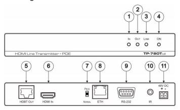
Figure 1: TP-780TXR HDMI Line Transmitter + POE
