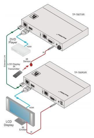
Figure 5: Controlling an LCD Display via the TP-780TXR/RXR
