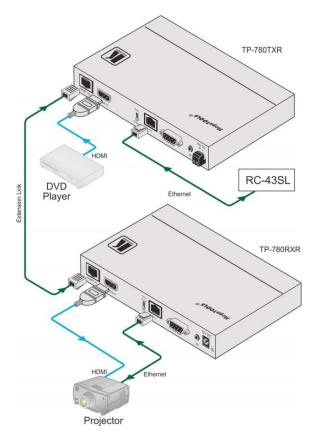
Figure 8: Ethernet Control via the TP-780TXR/RXR
