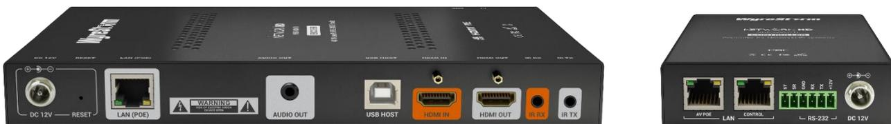
These units contain a network interface port that should be connected to a 1GbE link on a 1000BASE-T Ethernet switch with a cabling infrastructure that is suitable for use with IEEE 802.3ab standards with a link cable bandwidth tested to 100MHz across the entire link. This applies to the LAN ports on the Encoders, Decoders, as well as the AV/POE and Control ports on the CTL.
