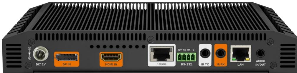
The 600 series contains a 10GbE SDVoE network interface port that must be connected to a 10GbE link on a 10GBASE-T Ethernet switch with a cabling infrastructure that is suitable for use with IEEE 802.3an standards with a link cable bandwidth tested to 500MHz across the entire link. This port is used for all AV over IP media streams between the TX and RX.
