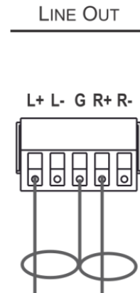
Figure 6: Connecting to an Unbalanced Stereo Audio Acceptor
