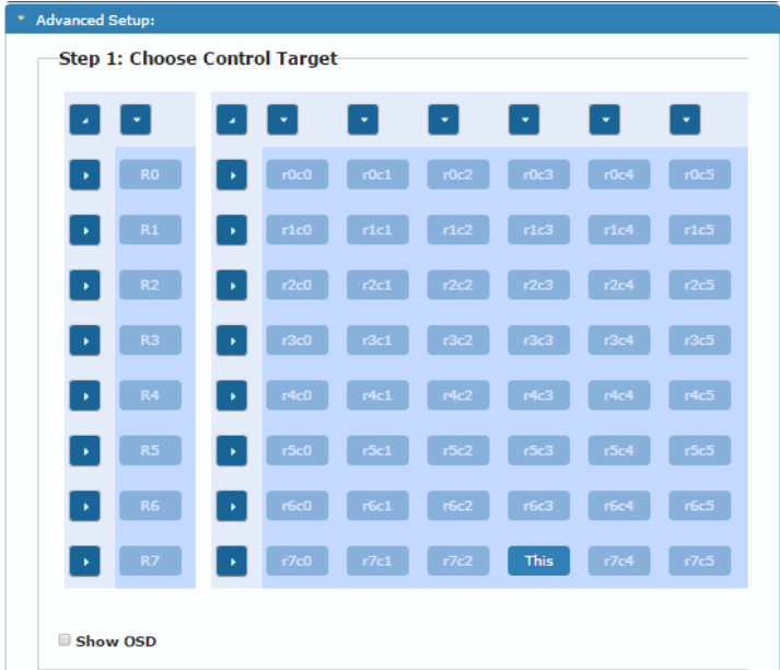
Figure 25: Video Wall Tab – Advanced Setup, Selecting a specific Device, Column or Row
