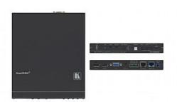
VP-428H2 is an HDBaseT 4K transmitter/scaler with HDMI, DP and VGA inputs. VP-428H2 supports HDBaseT tunneling of Ethernet, bidirectional RS-232 and IR signals, as well as PoE to provide power to the HDBaseT receiver. It receives the selected AV signal, up-scales, down scales or bypasses the video, according to the settings selected by the user, and converts it for sending via HDBaseT, together with the tunneled data and PoE
