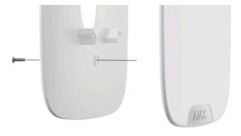
**11.** Fit the protective plastic panel in place (the Ajax logo on the connection side of the LED strip to the board) with little effort. The properly mounted plastic panel will protrude above the LED frame no more than 1.0 to 1.5 mm.
