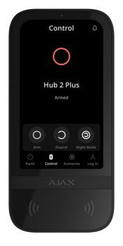
If Group Mode is enabled, users see the security mode of each group separately. The group is armed if its button outline is white and it is marked with  $\bigcirc$  icon. The group is disarmed if its button outline is grey and it is marked with  $\bigcirc$  icon.
