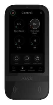
To instantly display the fire alarm muting screen on the KeyPad TouchScreen, enable the **Always Active Display** toggle in the KeyPad settings. Also, connect the third-party power supply.
