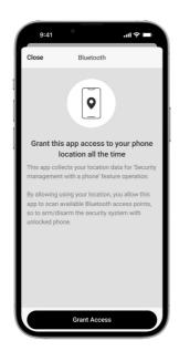
Bluetooth authentication can be unstable if **Geofence** function is disabled. You will need to launch and minimize the app if the system switches it to the sleep mode.
