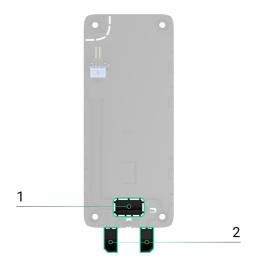
1 - to output the cable through the wall.
