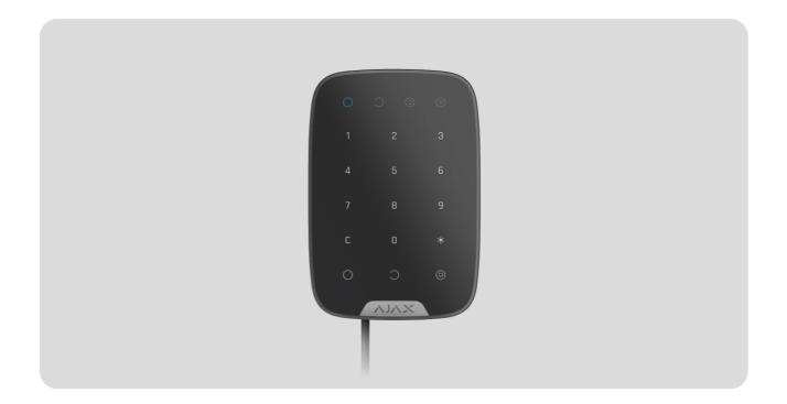
**KeyPad Fibra** is a wired touch keypad of the Ajax system. Controls the security modes and **Night Mode**. Supports duress code and protected from access code guessing. When it is active, the LED indication notifies about the security mode.
