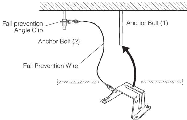
7. Attach one standard anchor nut to the Anchor Bolt (1), per illustration.
