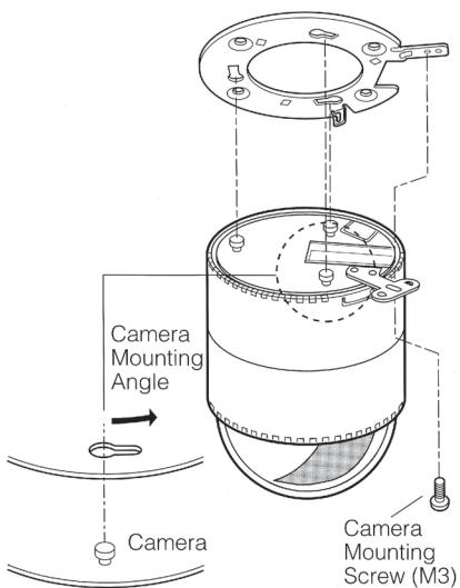
**Note:** When removing the Camera from the Camera Mounting Angle, loosen the Camera Fixing Screw (M3) and press up it by using the screw driver.
