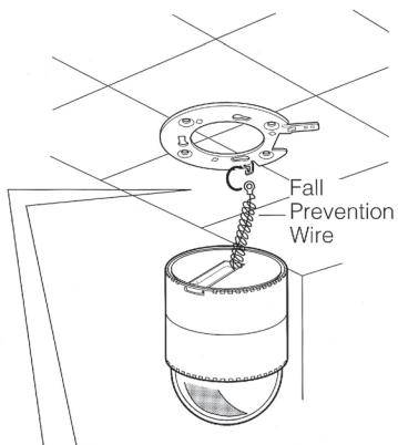
Be sure to match the wire with the Fall Prevention Wire Fixing Angle as shown below.
