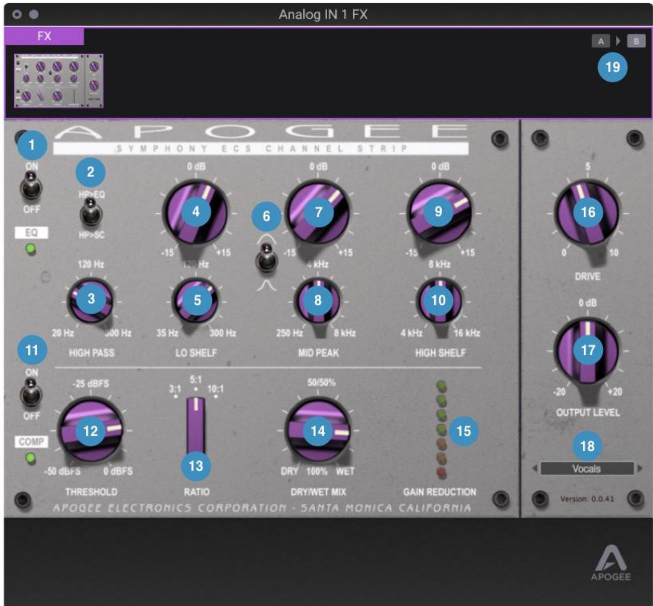
1. EQ Section In/Out - Toggle the EQ section on or off
