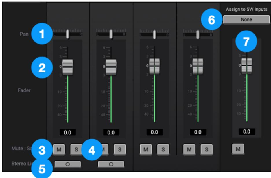
1. Channel Pan Control - Set the left-right placement of the channel signal in the mixer stereo output.
